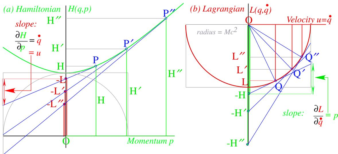
Fig. 5.1. Geometry of contact transformation between relativistic (a) Hamiltonian (b) Lagrangian
